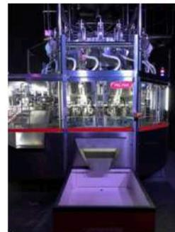
SC+ – High-speed HFFS machine. Photo – Volpak
