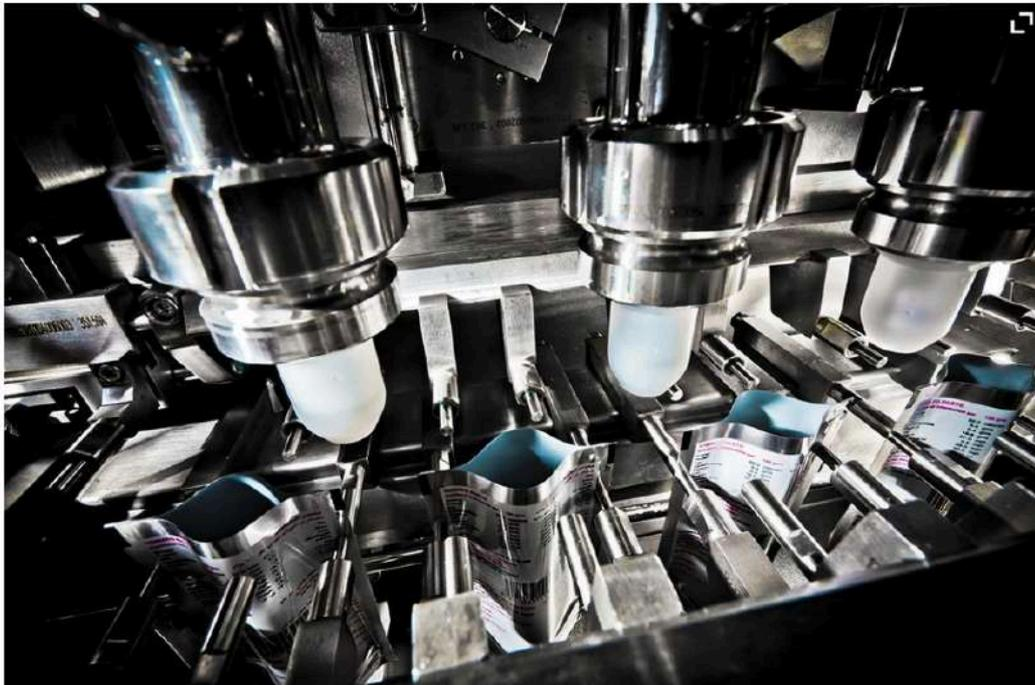
Volpak pouch horizontal form fill and seal equipment
