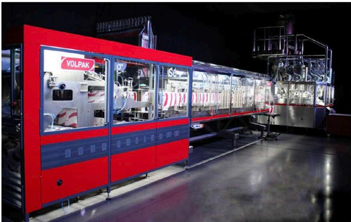
SC+ - High-speed HFFS machine. Photo - Volpak
